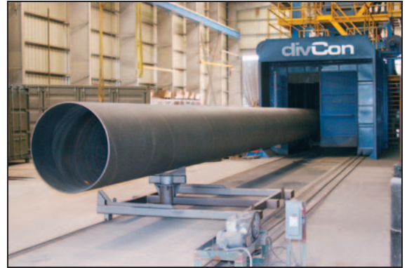
48" diameter x 85' pipe exiting wheel blast.
