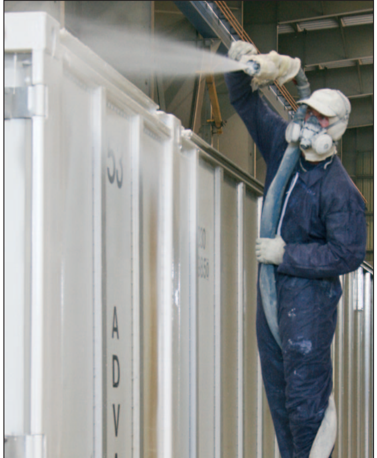
Application of Polyurea to ocean going steel shipping container.
