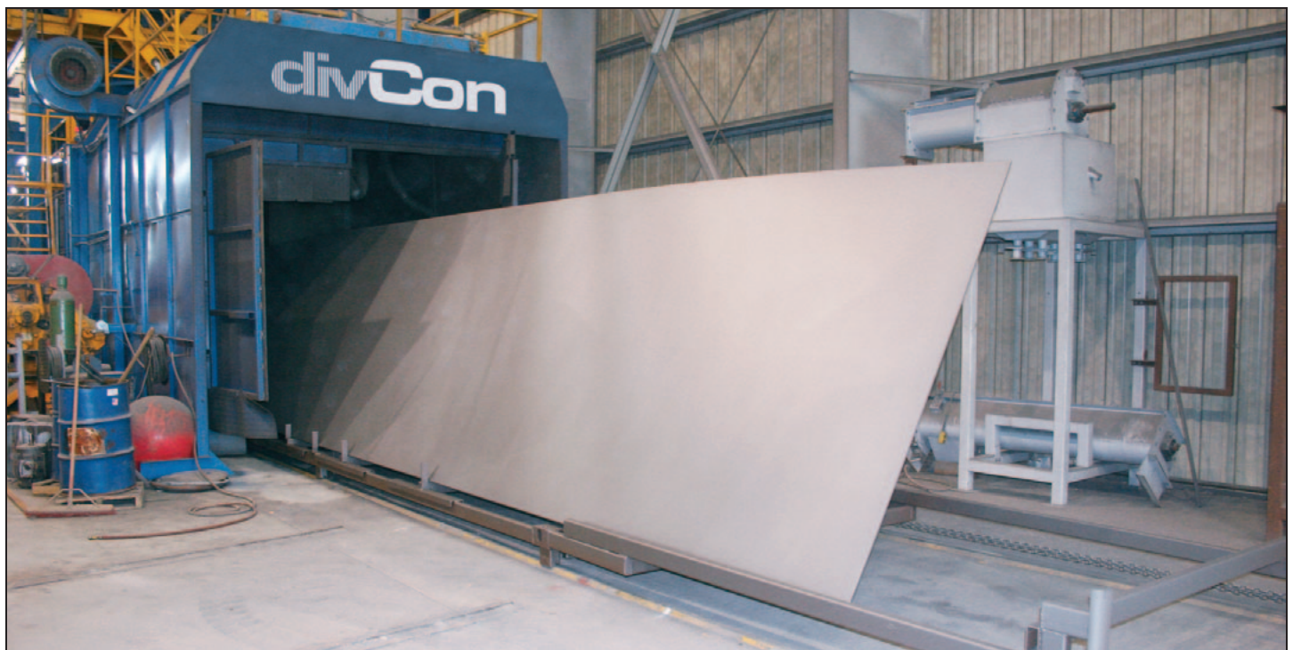
Descaled plate steel coated with pre-construction weldable primer.
