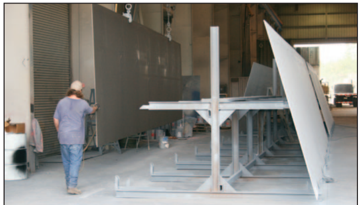
Descaled plate steel coated with pre-construction weldable primer.
